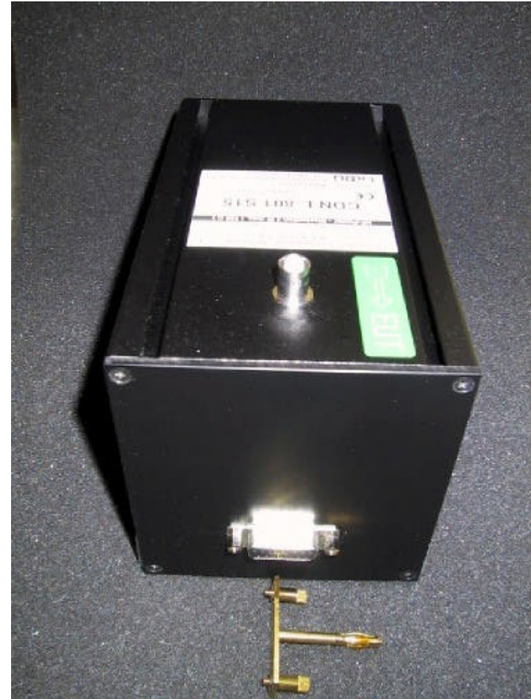
CDN Data 15 leads screened, D-sub 15 female
